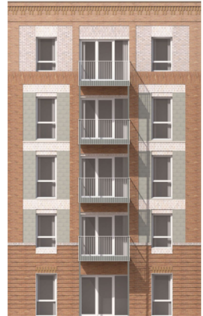
Typical bay elevation of building C
